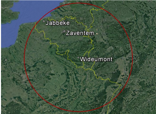
Fig. 3: Position of the 3 radar stations in Belgium and detection range of Wideumont radar station
