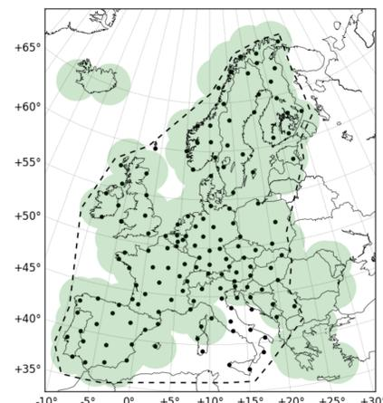
Fig: The locations of the EUCLID sensors are indicated as black dots, as well as an indication of the area within which EUCLID performs at its best by the dashed polygon. In addition, the collective detection range of the radars used within OPERA is indicated in green.
