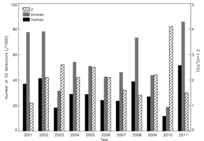
Figure 2. The amount of CG strokes (grey) and flashes (black) as detected by OP using a minimum of 2 sensors for a valid detection are plotted for each year. The ratio between CC flashes and CG flashes, Z, is plotted as well (/).
