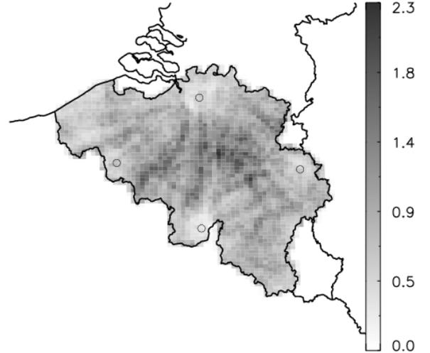
Figure 3. CG flash density (/km<sup>2</sup>/yr) averaged over 2001-2011. The open circles depict the positions of the 4 SAFIR sensors operated by OP.
