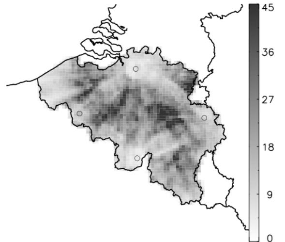
Figure 4. CC signal density (/km<sup>2</sup>/yr) averaged over 2001-2011. The open circles depict the positions of the 4 SAFIR sensors operated by OP.
