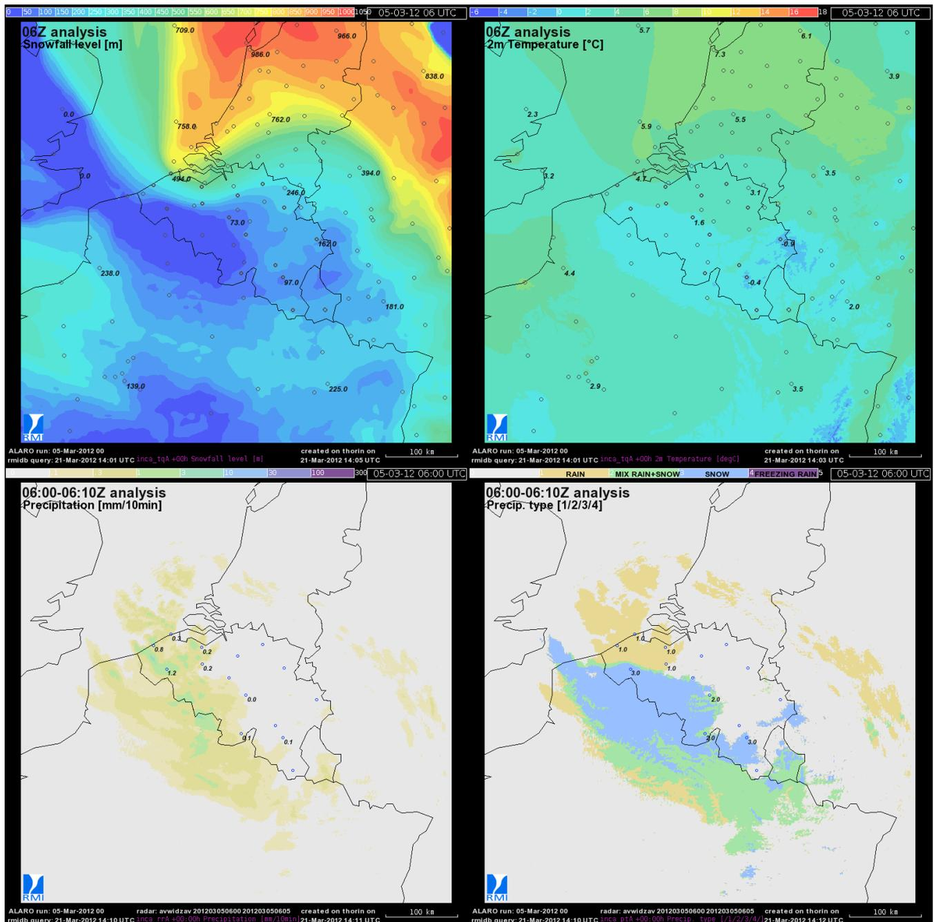
Figure 2: Snow case of March 05, 2012. The precipitation was caused by a low coming from the North Sea entering our country from the north of France. Upper left panel: snowfall level indicating the height of the snowfall layer; upper right panel: 2m temperature; lower panels: precipitation intensity (left) and precipitation type (right). Note the occurrence of snow while temperatures are slightly positive. All images are analysis fields at 06Z.
