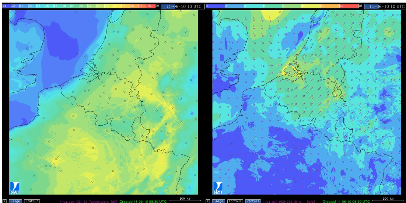
Figure 4: Examples of a 2m temperature (left) and 10m wind (right) forecast (+2h) generated by INCA-BE. This forecast is valid for 11-June-2010 at 10:00 UTC and was generated at 08:30 UTC, using station data recorded at 08:00 UTC, and using the NWP run of 00:00 UTC.
