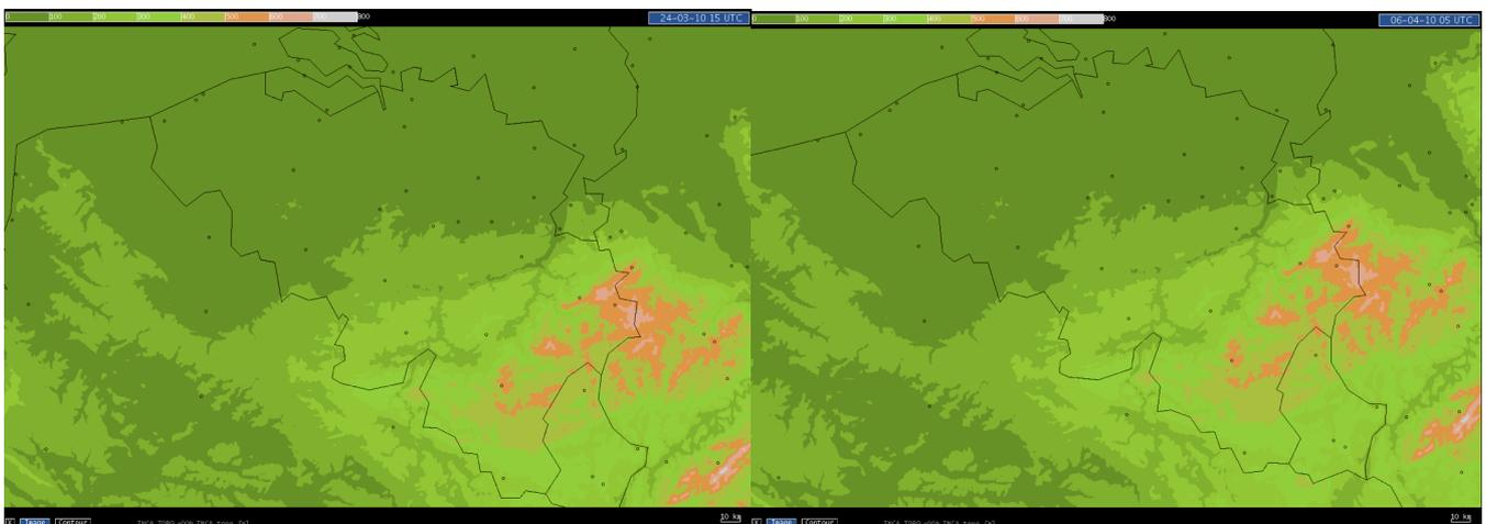
Figure 1: (Part of) the INCA-BE domain in two different projections. Left panel: the default INCA-AU projection which is a Lambert projection with a Bessel ellipsoid and centered on Austria; Right panel: the projection that we have chosen as the standard INCA-BE projection: a Lambert projection with a GRS80 ellipsoid and centered on Belgium.
