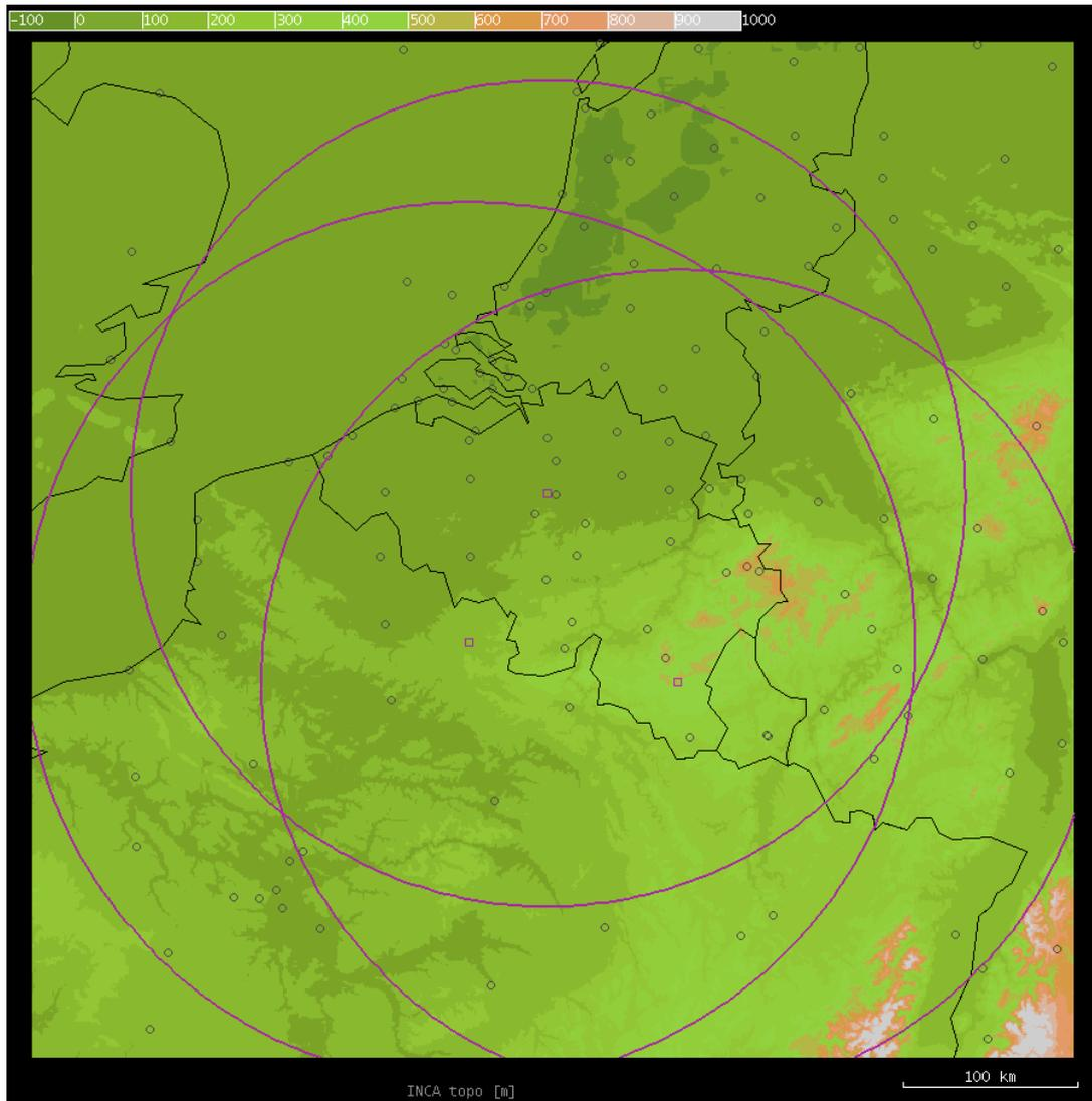
Figure 2: The INCA-BE topography generated by the INCA setup script. Superimposed are the positions of the radars and their ranges (purple squares and circles) for which we have data in near-real time, and the surface stations (small circles).
