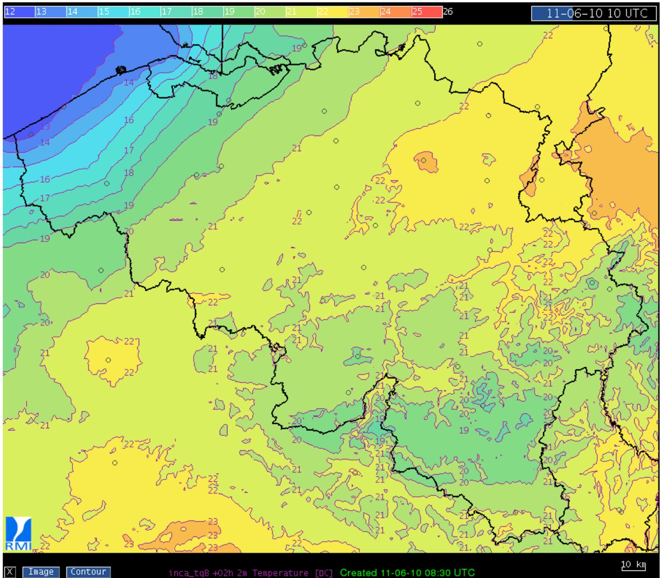
Figure 5: Zoom on Belgium for the 2m temperature forecast shown in Fig. 4. The colour scale of this figure slightly differs from the one in Fig. 4. Note the strong land-sea contrast, and the effect of the high-resolution topography, especially in the south of Belgium.
