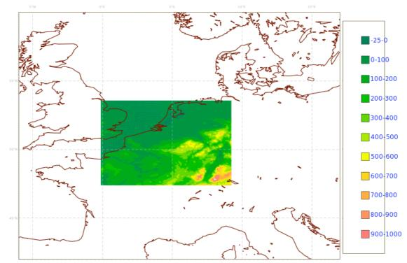
Figure 3: The domain of the NWP model (ALARO-0 4km) used in INCA-BE; the topography field (in m) is shown here.
